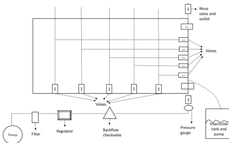
Fig. 2. Schematic design of 5 injection manifold (half of the design) and pump to deliver different treatments to individual plots
