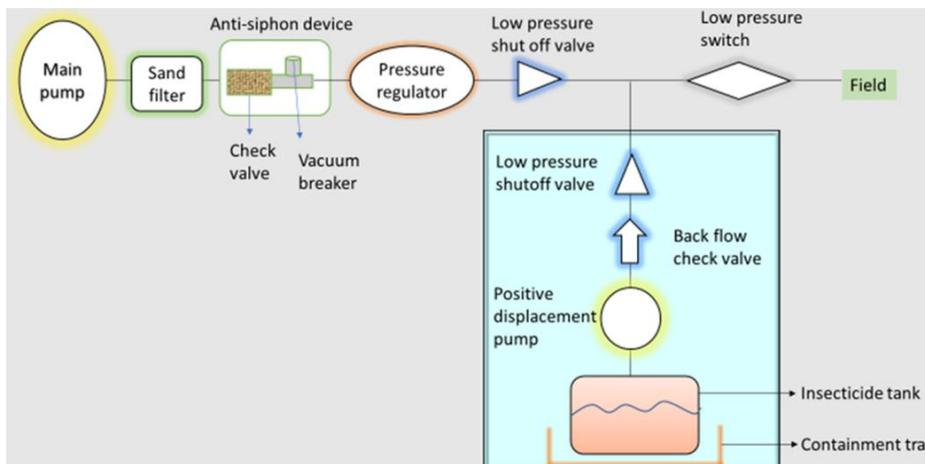
Fig. 1. Parts of insectigation equipment for the pre-existing drip system (Source: Ghidui, 2012)
